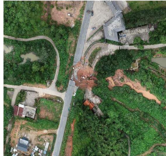
K32+220~K32+320 段路堤垮塌，护栏等防护设施损毁、浆砌拱涵崩塌
